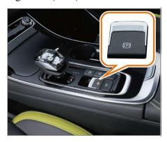
The driver can use the EPB switch to park the vehicle reliably.
