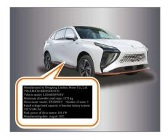
The vehicle sign is located under the right center pillar and contains the following information:
