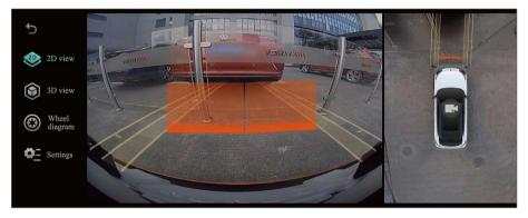
In the panoramic interface, when the working conditions of the radar system are met, the obstacle board will be displayed and an alarm sound will be given.
