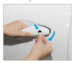
2. After the door is closed, pull the driver's door handle to the maximum opening, put the index finger into the handle and press the front clip, and take out the lock cylinder cover to expose the lock cylinder hole.
