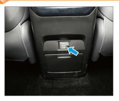
The rear USB interface is located below the rear air vent of the console.
