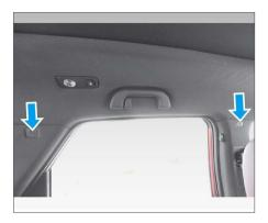
The side curtain SRS help protect the heads of the driver, the front passenger and the rear outboard passenger.
