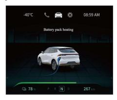
11. If the vehicle is slowly charged in a low-temperature environment and the traction battery heating system is turned on, if the charging power is too low, the A/C system cannot be used.
