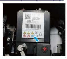
The battery warning mark is stuck to the surface of the battery. Remind you to keep the battery away from heat sources and open flames, and keep it ventilated
