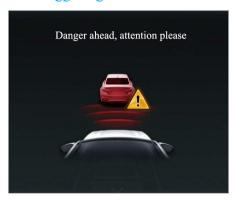
When the automatic emergency brake is triggered, the FCW system warning light on the instrument cluster flashes red, and the front of the driving interface is marked red. The text prompts [Danger ahead, please attention], accompanied by high-frequency alarm sound.
