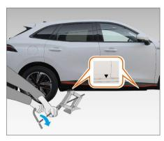
There are two jacking position identification points on the outer panels of the left and right doors respectively. Place the jack in the groove corresponding to the triangle mark point, and then jack up the vehicle.
