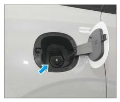
The AC charging port is located on the right rear side of the vehicle.
