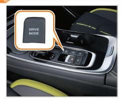
When the vehicle is started, the driving mode is "ECO" by default. Press the driving mode button once to switch to the "Normal" mode, and press this button again to switch to the "SPORT" mode.
