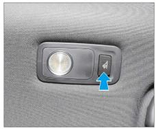
The rear interior lights are located below the rear handle. When the door control switch is parallel to the panel or "O" is pressed, the ON or OFF of the rear interior lights is controlled by the rear interior light switch.
