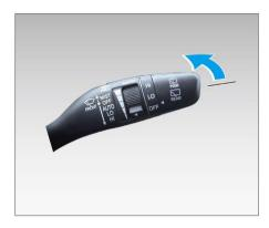
Push and hold the wiper control handle forward, and the rear windshield washer starts to spray water. At the same time, the rear wiper performs low-speed wiping. Release the wiper control handle to stop spraying water and wiping.
