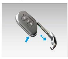
Press the mechanical key release button on the side of the smart key to take out the mechanical key.
