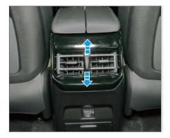
Roll the roller up and down to open and close the middle-row air vent, and move the grille in the middle of the air vent up and down, left and right to change the air direction.
