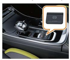
The AUTO HOLD function helps the driver to start the vehicle more comfortably on the slope section or at a traffic light intersection. This function can be activated and inactivated by press AUTO HOLD switch. After the function is activated, the system will continue to brake when the driver releases the brake pedal at the hill start or traffic light intersection.
