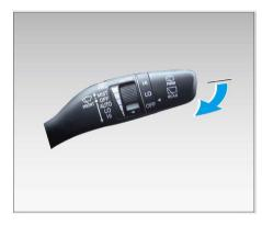
Pull back and hold the wiper control handle, and the front windshield washer starts to spray water, and the front wiper performs low-speed wiping at the same time. Release the wiper control handle and stop spraying water and wiping.
