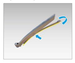
Check whether the wiper blades are worn or broken.
