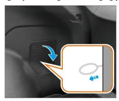
If the AC charging plug still cannot be pulled out after pressing the unlock button on the smart key or unlocking the door by carrying the smart key and holding the unlock area on the inner side of the driver's door handle, open the trunk lid, remove the right body maintenance hatch cover and pull out the emergency unlocking tab for a certain distance to unlock the AC charging plug in an emergency.
