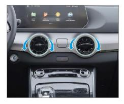
Turn the air vent switch knob clockwise to close the air vent, and counterclockwise to open the air vent. The air direction can be changed by moving the grille in the middle of the air vent up and down, left and right.
