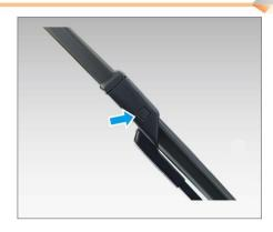
1. After activating the wiper maintenance mode, pull up the wiper arm, pull out the wiper blade along the opening direction of the wiper rod, and remove the wiper blade.
