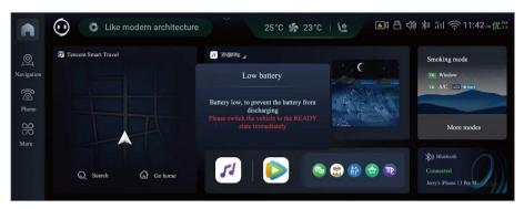
When the vehicle is not switched to READY status, if the system detects that the 12 V low-voltage battery power is less than 60%, a text window will pop up on the display, suggesting that the 12 V low-voltage battery power is too low, at this time, you should immediately switch the vehicle to READY status, and recharge the 12 V low-voltage battery, or it may affect the normal use of the vehicle. This reminder will be automatically dismissed after the vehicle is switched to the READY status.
