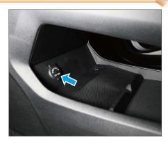
The front 12 V on-board power supply is located in the storage tank at the lower storage slot of the console.
