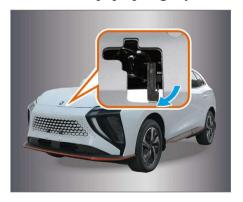
2. Pull the safety lock lever to the left and lift the hood.
