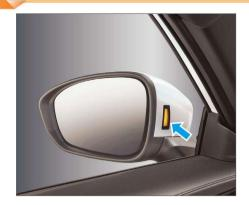
The warning lights are located at the mirror housings of the left and right exterior rearview mirrors.
