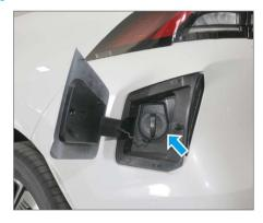
The DC charging port is located on the left rear side of the vehicle.
