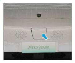
The DC charging port is located right in front of the vehicle.
