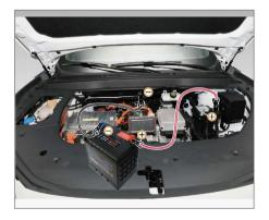
6. As shown in the figure, avoid the 12 V low-voltage battery and moving parts, and connect the clip on the other end of the negative cable to a solid, fixed, unpainted metal part of the host vehicle.
