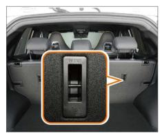
4. Pass the hook of the child safety device through the seat headrest, fasten it to the fixed anchor support on the back of the seat, and tighten the top tether to ensure that it is fastened firmly.
