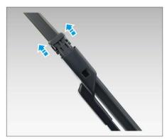
2. Replace the wiper blade with a new one, and operate in the reverse order to ensure that the wiper blade is correctly installed in place.
