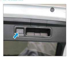
Press the trunk lid shield switch to automatically close the trunk lid. If this switch is pressed again during closing, the trunk lid will stop closing.
