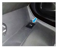
Type-C power interface is located in the lower storage slot of the console and supports the charging of mobile phones, tablets and laptops (the charging equipment interface shall be a Type-C interface).
