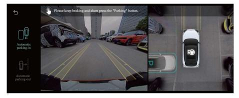
After identifying the parking space the driver parks the car and activates the auto-parking by short press on the parking button according to the prompts, releasing the steering wheel and brake, the vehicle starts to park automatically.
