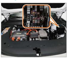
The engine compartment fuse box is located at the upper left part of the engine compartment. Remove the clips on the left and right sides of the fuse box, and open the box cover to check the fuse.
