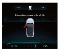
This interface displays some vehicle information that needs to be alarmed or reminded. When there are multiple vehicle information that need to be alarmed or reminded, the displayable content can be switched and inquired by pressing the UP and DOWN buttons on the steering wheel.
