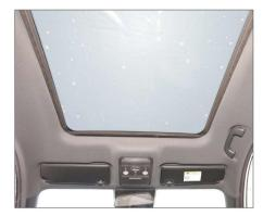
The panoramic glass roof is made of integral glass and cannot be opened. The panoramic glass roof of some models has starry patterns.
