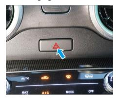
Press the hazard warning light switch above the A/C control panel, and the turn signal and the turn signal and hazard warning light on the instrument cluster will start to flash to remind pedestrians and passing vehicles to avoid the vehicle.
