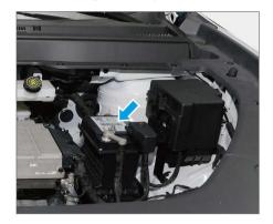
This vehicle is equipped with a maintenance-free 12V low-voltage battery, which is located on the left side of the engine and mainly provides electric energy for vehicle starting and on-board electrical appliances. If the 12V low-voltage battery is seriously undervoltage, the vehicle will not be able to start.
