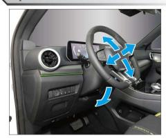
After holding the steering wheel with one hand and pulling the adjustment handle downward with the other hand, you can move the steering wheel horizontally and vertically to adjust it to the desired position. After adjustment, pull up the adjustment handle and confirm that it is locked in place.
