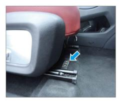
1. It is engraved on the body crossmember under the front passenger seat and can be seen by lifting the carpet gap.
