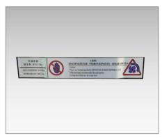
The radiator warning label and the A/C refrigerant label are pasted above the inner side of the hood. When replacing the coolant, use the coolant specified by Dongfeng Forthing. Do not mix coolants of different brands. Do not touch the radiator, as the cooling fan may rotate at any time.
