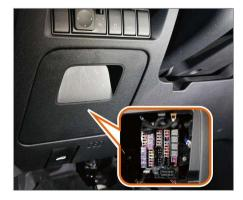
The interior fuse box is located in the lower left corner of the dashboard. Remove the cover plate to check the fuse.
