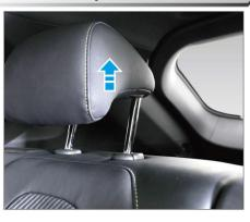
3. Raise the headrest to the highest point until you hear a "click" sound, so as to ensure that the headrest is locked in place.
