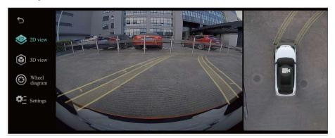
There are auxiliary lines in the 2D front and rear single view (middle) and 2D splicing view (right). The auxiliary lines switch between the front and rear directions with the switching between D gear and R gear. The actual length indicated by the auxiliary lines is 5m.
