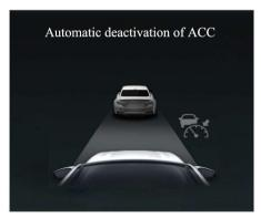
Under certain driving conditions, the deceleration capacity of the ACC system is not enough to keep a sufficient distance from the vehicle ahead, and the ACC system will require the driver to take over the vehicle in time.
