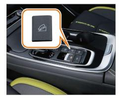
Press the HDC switch, and the hill descent control system working indicator light on the instrument cluster will illuminate, indicating that the HDC system is turned on. When the HDC switch is
