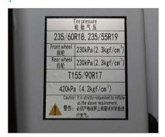
Tire pressure labels are attached on the vehicle. This label is located below the driver's door frame and indicates the air pressure of the front and rear wheels of the vehicle.
