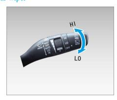
HI: High-speed wiping of rear wiper. Turn the rear end of the wiper control handle to the HI position, and the rear wiper performs 05
