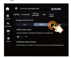
Glide energy recovery has the effect of braking and deceleration, and you can set the glide energy recovery to one of the three gears - low, medium and high - according to your driving habits. This gear can be memorized automatically. In the gear with weak coasting energy recovery, energy recovery will not be carried out (if
