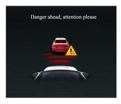
The level I alarm will be triggered when the vehicle may be in danger of collision. The warning light of the FCW system on the instrument cluster flashes in red, and the front part of the driving interface is marked in red. The text prompts [Danger ahead, attention please], accompanied by medium-frequency alarm sound.
