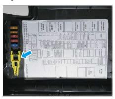
There is a fuse puller in the engine compartment fuse box. Pull the fuse straight out of the fuse box with the puller. If the fuse is not blown, there must be other causes causing the fault. Please contact an authorized service station of Dongfeng Forthing as soon as possible.
