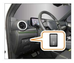
The ESP system is turned on by default. Press the ESP switch to turn off the ESP system, and the ESP OFF indicator light on the instrument cluster will illuminate.
