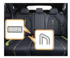
1. Locate the ISOFIX interface in the gap between the rear seat cushion and the backrest.
