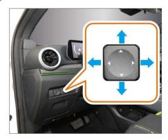
Move the mirror adjustment switch up, down, left and right to adjust the exterior rearview mirror to the best view angle.
