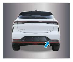
If the vehicle needs to be towed, please contact the professional vehicle towing service department. Do not tow the vehicle only with ropes or iron chains.
