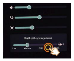
3. Slide the control ball leftward or rightward to adjust the headlight height. There are four levels.
