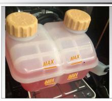
Check whether the coolant level is between the upper limit (MAX) and the lower limit (MIN) scale marks. If it is lower than the lower limit, add coolant to the coolant expansion tank to the position near the upper limit.
