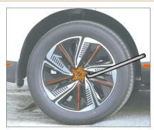
Remove the wheel nuts with a wheel nut wrench, and then remove the tire.
