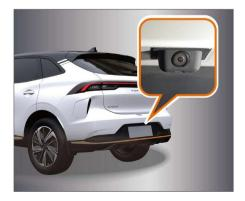
The reversing camera collects images through the camera installed behind the vehicle, which is convenient for the driver to check the obstacles behind in time when reversing.
