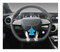
The horn is located in the middle of the steering wheel. Pressing the horn can remind pedestrians and vehicles outside the vehicle. Reasonable use of horns will help to ensure driving safety and reduce the frequency of accidents.
