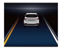
When the vehicle may deviate from the lane, slightly turn the steering wheel to correct the vehicle to return to its own lane. The driving interface of the instrument cluster deviates from the lane line and turns yellow.
