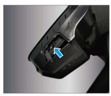
The memory card slot of the vehicle traveling data recorder is located on the left side of the vehicle traveling data recorder. Please confirm whether there is a memory card in the card slot before the first use.
