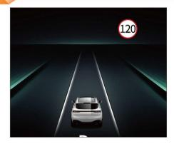
When the vehicle passes by a speed limit sign, the instrument cluster will display the speed limit sign. When the vehicle is overspeed, the speed limit sign on the instrument cluster flashes and disappears after 10 seconds or below the speed limit.
