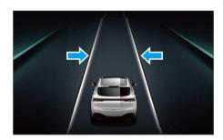
Short press the "Lane keeping" button to activate the function, and the working indicator light of the LKA system on the instrument cluster illuminates in white. If the system detects lane lines and the activation speed is met, the lane lines on both sides will turn white.
