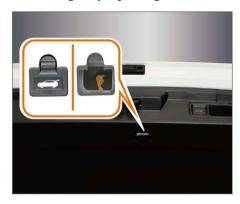
If the lock fastener fails and the trunk lid cannot be opened, remove the emergency opening cover plate from the trunk lid shield, pull the emergency opening pull ring of the trunk lid, and hold the trunk lid backward with the other hand to open the trunk lid from inside the vehicle.
