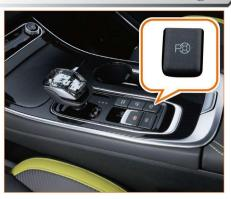
When the vehicle speed is below 30 km/h, press the full automatic parking switch to enable the parking-in function.
