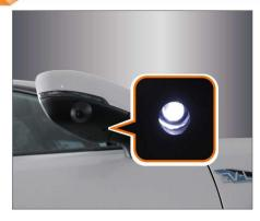
The courtesy light is located below the exterior rearview mirror of the vehicle and used to illuminate the ground at night. When the door is opened, the courtesy light will light up; after the vehicle power supply is turned off, when the door is pushed open, the courtesy light will light up; after the door is closed, the courtesy light will go out.
