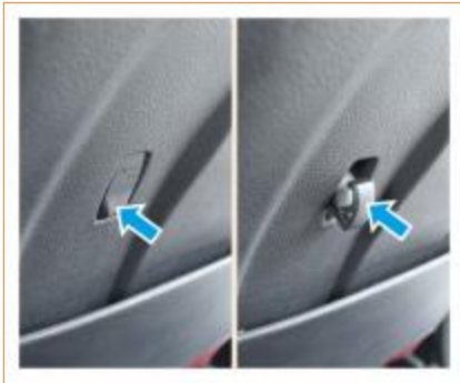
The front seat backs are designed with hooks for hanging lightweight items such as cups of water.
