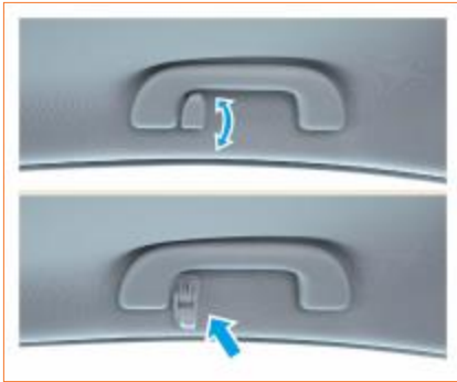
Rear right hand interior handle with coat hooks for passenger use
