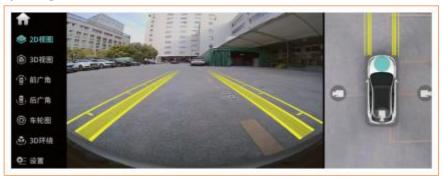
There are dynamic guide lines in 2D front and rear single views and the splicing view. The forward and backward directions of the dynamic guide lines switch with the switching of D and R gears, and the actual distance indicated by the guide lines is about 5 m.
