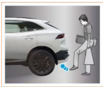
The foot-activated sensor is located below the middle of the rear bumper. To open the trunk lid, kick at the position shown in the figure. After a sound signal is heard, the trunk lid will open automatically and the turn signals will flash.
