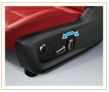
Push the upper part of the backrest angle adjustment button forward or backward gently to adjust the seat backrest angle forward or backward.
