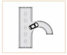
When the vehicle runs to an expressway ramp, the TJA system may exit due to a reduced speed lower than the effective one when entering the ramp or recognition of excessive ramp curvature or unclear lane line.
