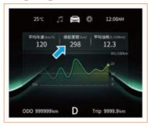
The endurance mileage is estimated based on the latest comprehensive fuel consumption and the remaining amount of fuel in the fuel tank, and it means the maximum mileage that can be continued from now on.
