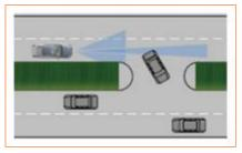
When the target vehicle followed by the subject vehicle makes a U-turn or right-angle turn, the sensor will lose the target and the system may accelerate automatically. The driver shall continuously pay attention to the surrounding environment and be ready to take over at any time.
