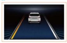
The left lane departure warning is sent, the departed lane line turns red in the main interface, and the buzzer gives an alarm.
