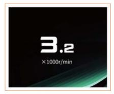
The tachometer displays the number of engine revolutions per minute (×1,000 r/min). To prevent damage to the engine, do not drive at a speed in the red number zone for a long time.
