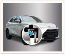
2. Move the safety lock lever in front of the engine hood leftward with fingers, and lift up the engine hood.
