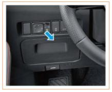
The interior fuse box is located at the lower left corner on the driver's side. Remove the cover plate to check the fuse.
