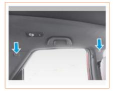
The side curtain airbags are installed above the left and right doors in the vehicle, marked with "SRS AIRBAG" (for some models). Side curtain airbags help to protect the heads of the driver, the front passenger, and the rear outer passenger.
