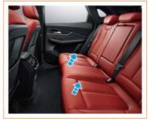
Lift the front end of the seat cushion with force, pull it forward to a position where its front end contacts the front seat backrest, and then turn over the seat cushion so that its front end faces downward to contact the floor and form an angle approximately perpendicular to the floor.
