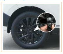
Take out the wheel nut cap clip from the clamping foam, and take out the nut trim cover with the wheel nut cap clip.
