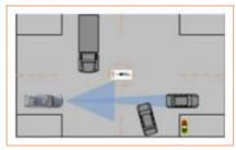
When the target vehicle followed by the subject vehicle passes through an intersection, the driver shall pay attention to the change of traffic lights and take over the vehicle when necessary to avoid violating traffic rules.
