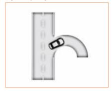
When the vehicle runs to an expressway ramp, the LKA system may exit due to a reduced speed lower than the effective one when entering the ramp or recognition of excessive ramp curvature or unclear lane line.
