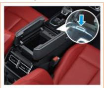
A central storage bin is designed under the front-row central armrest. Press the front button of the central armrest to open the central storage bin automatically.
