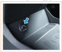
The 12 V on-board power supply is located above the lower storage tank of the console. It can work only when the Start/Stop switch is set to "ON" or "ACC".
