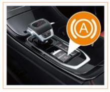
The AUTO HOLD function can help the driver to start more comfortably on a slope or at an intersection with traffic lights. This function can be turned on or off by AUTO HOLD switch. After the AUTO HOLD function is turned on, if the driver releases the brake pedal when starting on a slope or at an intersection with traffic lights, the system will continue to hold braking.
