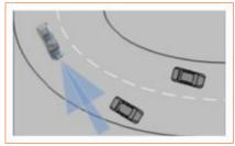
When the followed target vehicle leaves the expressway or turns, the TJA system will lose the target and may accelerate automatically.
