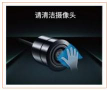
When the camera needs to be cleaned, the combination instrument will display a prompt message.
