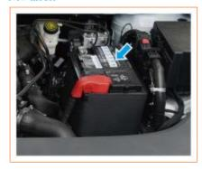
The vehicle is equipped with maintenance-free battery. The battery is located on the left side of the engine compartment, which mainly provides electric energy for vehicle starting. If the battery is seriously depleted, the vehicle will fail to start.
