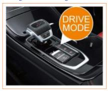
The vehicle starts in Normal mode by default. When the driving mode button is pressed for the first time, it switches to SPORT mode, and when it is pressed for the second time, it switches to ECO mode. Press the driving mode button to realize cycle switching between Normal  $\rightarrow$  SPORT  $\rightarrow$  ECO  $\rightarrow$  Normal.
