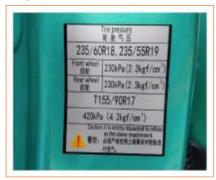
Tire pressure labels are attached on the vehicle. The label is located below the door frame on the driver's side, indicating the front and rear tire pressure and spare tire pressure of the vehicle.
