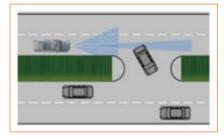
When the target vehicle followed by the subject vehicle makes a U-turn or right-angle turn, the sensor will lose the target and the system may accelerate automatically. The driver shall continuously pay attention to the surrounding environment and be ready to take over at any time.
