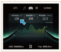
This interface displays the average vehicle speed after the last resetting. Display range:  $0{\sim}200$  km/h.
