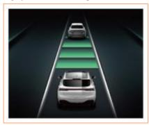
When the following distance is set to be long, the combination instrument displays as shown in the figure above.
