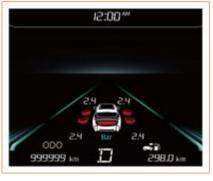
The interface displays the pressure value corresponding to the tire. In case of any tire abnormality, the display interface will give a corresponding reminder.
