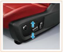
Push the seat forward/backward/height adjustment button upward or downward gently to raise or lower the seat as a whole.
