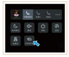
Swipe down on the multimedia display screen, tap "Rearview Mirror Folding", or tap [Settings]-[Vehicle]-[Accessories] on the screen in sequence to enable [Automatic Folding of Exterior Rearview Mirror] function, and then the rearview mirror can be folded and unfolded electrically.
