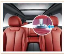
To raise or lower the headrest, press the adjustment switch on the side of the seat headrest, lift up or press down the headrest to the desired height, and then release the switch. Press down or lift the headrest slightly again until a click is heard to make sure the headrest is locked in place.
