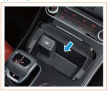
A storage box is designed on the upper part of the console. Press the storage box cover to open it, and some small objects such as mobile phones can be placed inside.
