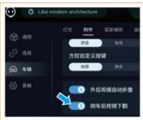
Tap [Settings]-[Vehicle]-[Accessories] on the display screen in sequence to enable the [Reversing rearview mirror tilt-down] function. When the vehicle is reversing, the exterior rearview mirror can automatically tilt down for a certain angle in order to help the driver check the road conditions.
