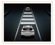
When the following distance is set to be ultra-long, the combination instrument displays as shown in the figure above.
