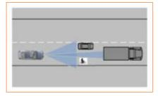
The ACC system cannot detect all types of vehicles on the driving path, especially
