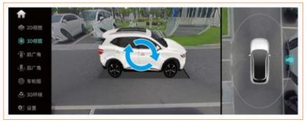
Tap "3D View" on the left to enter the 3D view interface. Drag the icon of the splicing area to rotate 360°, and it is also possible to zoom or drag the interface.
