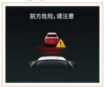
When the FCW system is triggered, a warning icon will be displayed in the combination instrument pop-up box and an audible alarm signal will be given at the same time.
