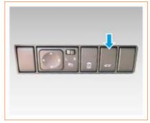
With the trunk lid closed, press the trunk lid switch on the instrument panel switch set to open the trunk lid automatically.
