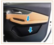
The interior trim panels of the front and rear doors are designed with door storage boxes for storing cups and other articles.
