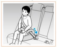
Place the auxiliary cushion on the seat and let children sit on the auxiliary seat cushion. According to the manufacturer's instructions, thread the seat belt over children's shoulder, lower the lap belt as low as possible to children's buttock position, and then insert the locking tab into the buckle to ensure the seat belt is not twisted and kept taut.
