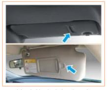
A ticket holder is designed on the sun visor, which can be used to place small items such as invoices and refueling cards.
