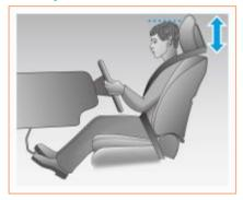
Adjust the height of the headrest to make its top not lower than the top of the driver's head, which can reduce the risk of neck injury in case of emergency braking.
