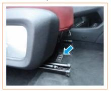
1. It is engraved on the body crossmember under the front passenger seat and can be seen by lifting the carpet gap.
