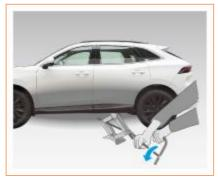
Before jacking the vehicle, place a chock in front of and behind the wheel diagonal to the tire to be replaced, and then use a wrench to unscrew the wheel nut to be replaced by half a turn.
