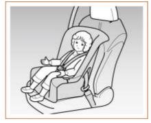
According to the weight and height requirements specified by the manufacturer of CRS, children over one year old should use forward-facing CRS when riding in the vehicle.
