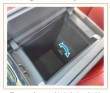
The central storage bin is designed with a vent, and the vent can be opened or closed by turning the switch.
