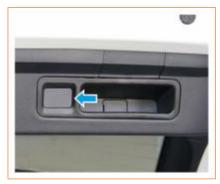
Press the trunk lid shield switch, the trunk lid will be closed. Press this switch again in the process of closing, the trunk lid will stop closing.
