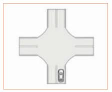
When the vehicle travels to an intersection, the TJA system may exit due to absence of the lane line ahead, or abnormal identification and steering may occur due to the influence of crosswalk and other road markings at the intersection.
