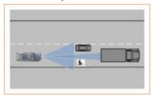
The TJA system cannot detect all types of vehicles on the driving path, especially narrow vehicles such as electric vehicles, bicycles and motorcycles, or vehicles with high chassis and loads exceeding the body. The driver shall pay close attention to the surrounding environment of the vehicle.
