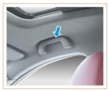
Interior handles are provided on both sides of the front and rear rows for passengers to use under special circumstances. The interior of the door handle is equipped with a spring mechanism, which automatically returns to its original position when released.
