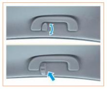
The interior handles on both sides of the rear row are provided with coat hooks (for some models, only the rear right handle is equipped with one) for passengers to use.
