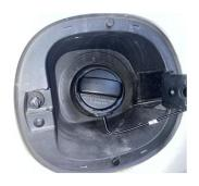
Rotate the fuel filler cap counterclockwise to slowly open it and add fuel. After refueling, rotate the fuel filler cap clockwise until a click is heard, indicating it is closed.
