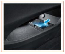
The wireless charging device is located in front of the lower storage tank of the console. It can be used to charge portable chargeable devices (such as mobile phones) that support wireless charging.
