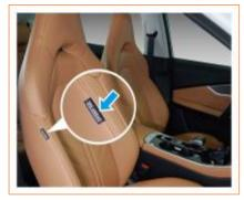
The front side airbag helps to protect the torso of the driver and front passenger from the impact of interior components.
