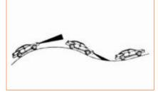
Do not use the ACC system when the vehicle is running on a bumpy slope. On a bumpy slope, the ACC system cannot detect vehicles on the same lane and will automatically turn off when the driver depresses the brake pedal frequently.
