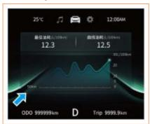
The fuel consumption curve is drawn based on the curve fuel consumption within the last 50 km. This information can help you adjust your driving habits to achieve the expected fuel consumption.
