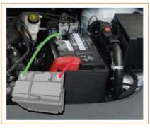
If the vehicle cannot be started due to low battery, jumper cables can be used to start with the help of batteries on another vehicle. Jumpering is dangerous and should be operated with caution.
