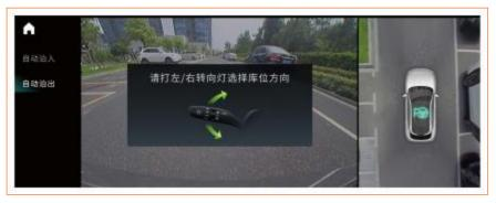
2. After selection, the driver releases the steering wheel and the automatic parking system starts horizontal parking-out. Parking-out process
