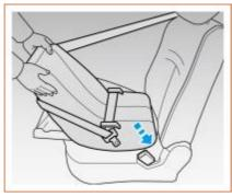
According to the manufacturer's instructions, thread the seat belt through or around the rear-facing CRS. Then, insert the locking tab into the buckle, ensuring the seat belt is not twisted and remains taut. Confirm that the locking tab and buckle are locked securely, and check the stability of the CRS by shaking it from side to side.
