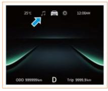
This interface displays driving information, driver assistance, multimedia, map navigation and settings. The display content can be switched by pressing the left and right buttons on the steering wheel.
