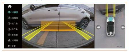
Radar obstacle board display: In the panoramic interface, when the working conditions of the radar system are met, the obstacle board will be displayed and an alarm sound will be given.
