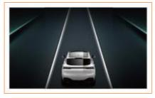
When no lane line is detected, no lane line is displayed on the main interface.
