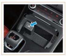
The front USB interface is located in the upper storage box of the console. Press the storage box cover to open it for use. It can only work when the Start/Stop switch is set to "ON" or "ACC".
