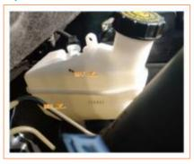
Check the fluid level in the fluid reservoir once a month. Check whether the brake fluid level is between the upper limit (MAX) and lower limit (MIN) marks. If the fluid level is at or below the lower limit (MIN) mark, check whether the brake system leaks and whether the brake pads are seriously worn.
