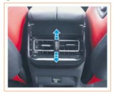
Roll the roller up and down to open and close the rear-row air outlet, and move the grille in the middle of the air outlet up and down, left and right to change the air direction.
