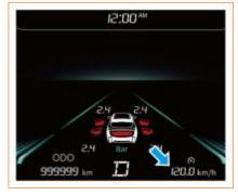
This interface displays the average vehicle speed after the last resetting. Display range: 0~200 km/h.
