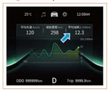
This interface displays the average fuel consumption after the vehicle is reset last time, with display range of 0~19.9 L/100 km.
