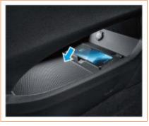
A storage tank is designed at the lower part of the console for placing some small items, such as mobile phone and keys.
