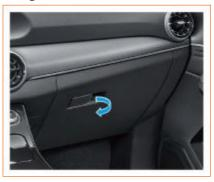
The storage box is located on the front passenger side. Pull the storage box cover handle backward to open the storage box. Push back the storage box cover forward and buckle it to close the storage box.
