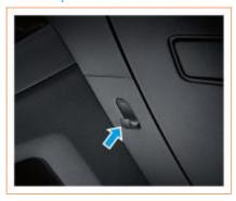
The left side of the storage box is designed with a hook, which can hang light items such as cups. Press the groove to open it, and press the convex rib to close it.
