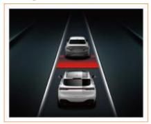
When the following distance is set to be short, the combination instrument displays as shown in the figure above.
