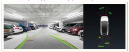
The left picture is the reversing image, and the right picture is the reversing radar \*. There are three safety levels: green, yellow and red according to obstacles from far to near.
