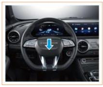
The horn switch is located in the middle of the steering wheel. Pressing the horn switch can remind pedestrians and other vehicles to reduce accidents. Reasonable use of the horn helps ensure driving safety.
