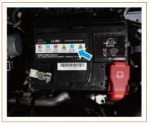
The battery warning mark is stuck to the surface of the battery. The battery shall be kept away from heat sources and open
