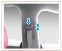
After pressing the upper part of the shoulder belt height adjuster to move the adjuster up and down to the desired position, try to move the adjuster down without pressing to make sure that it is locked in place.
