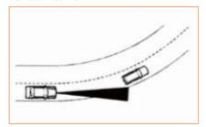
When the vehicle is in a curve, the ACC system may not be able to detect vehicles ahead on the same lane and the driver may lose control of the vehicle or have an accident. Please pay close attention and be ready to take over at any time.
