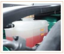
Check whether the coolant level is between the upper limit (MAX) and lower limit (MIN) marks. If it is below the lower limit mark, add coolant to the coolant reservoir until the upper limit mark.
