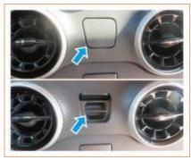
A mobile phone holder interface is arranged in the middle of the instrument panel, which is convenient for use during driving.
