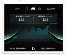
This interface displays the fuel consumption within the last 50 km. It includes optimal fuel consumption, curve
