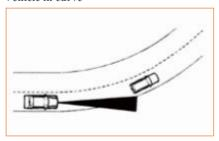
When the vehicle is in a curve, the TJA system may not be able to detect vehicles ahead on the same lane and control the vehicle accurately. Please pay close attention and be ready to take over at any time.
