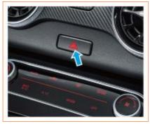
Press the hazard warning switch above the A/C control panel to turn on the hazard warning light. At this time, all turn signals outside the vehicle and the turn signal and hazard warning indicators on the combination instrument will flash to remind pedestrians and passing vehicles that the vehicle is in an abnormal state.
