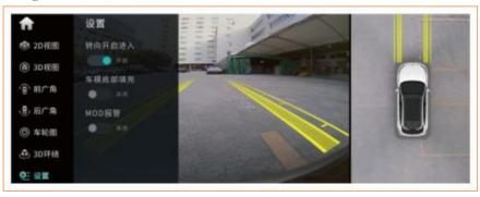
Functions such as entering when steering ON, bottom filling of vehicle model and MOD alarm can be turned on and off in the settings.
