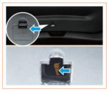
If the lock actuator fails and the trunk lid cannot be opened, first remove the emergency opening cover plate on the inner shield of the trunk lid, push the emergency opening handle of the trunk lid lock to the left, and press the trunk lid backward with the other hand at the same time to open the trunk lid from inside.
