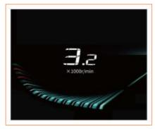
The tachometer displays the number of engine revolutions per minute (×1,000 r/min). There is a dynamic speed display bar below the digital display. To prevent damage to the engine, do not drive at a speed in the red zone.
