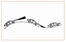
Do not use the TJA system when the vehicle is running on a bumpy slope. On a bumpy slope, the TJA system cannot detect vehicles on the same lane and will automatically turn off when the driver depresses the brake pedal frequently.
