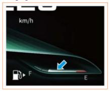
The fuel gauge displays the amount of fuel in the fuel tank in energy block. When the vehicle is turning or running on an uneven road section, the displayed fuel level will slightly deviate from the actual value. If the fuel quantity is small, the low fuel level warning indicator lights up to show that the fuel level in the tank is insufficient and that refueling has to be done as soon as possible.
