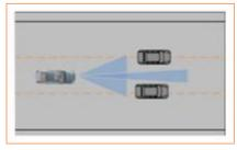
The ACC system cannot accurately judge the width of the lane ahead. When feeling that it is impossible to pass through normally, the driver shall immediately depress the brake pedal to turn off the ACC system and take over the vehicle.
