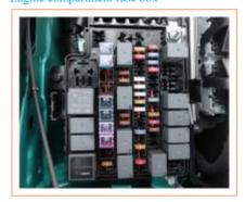
The engine bay fuse box is located on the left front side of the engine compartment. Remove the clips on the left and right sides of the fuse box, and open the box cover to check the fuse.
