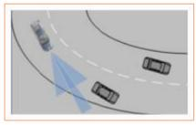
When the followed target vehicle leaves the expressway or turns, the ACC system will lose the target and may accelerate automatically.
