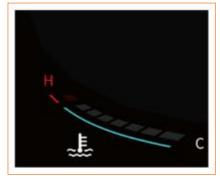
The coolant thermometer indicates the current engine coolant temperature. When the scale is close to H, the high coolant temperature warning indicator ... lights up, indicating that the engine is overheated at this time. Please park the vehicle in a safe
