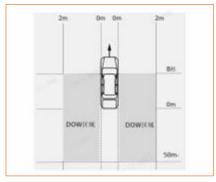
The alarm area of the DOW system is 0 m to 2m laterally from the left and right sides of the vehicle, and longitudinally from B-pillar to 50 m behind the rear of the vehicle, as shown in the figure. The shaded area is the warning area, which is bilaterally symmetrical.
