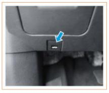
1. Pull the engine hood opening handle under the left instrument panel, and the engine hood will pop up slightly.
