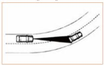
When the vehicle is entering/leaving a curve, the TJA system may respond to vehicles on adjacent lanes and apply brake. This braking process can be ended in advance by depressing the accelerator pedal.
