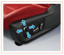
Gently press the forward, backward or upward and downward position of the backrest and lumbar support adjustment button (for some models, it can only be adjusted forward and backward) to adjust the position of the lumbar support. After adjusting to a proper position, release the button.
