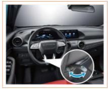
Adjust the steering wheel up, down, forward and backward to a proper position by adjusting the adjustment handle on the steering column. After adjustment, make sure that the adjustment handle is fully locked.
