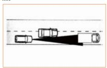
For a vehicle that is not running in the same straight line (a vehicle entering from the adjacent lane), if they do not enter the detection range of the camera sensor, the sensor may not detect that vehicle, resulting in ACC response delay. The driver shall pay close attention to the movement of vehicles in adjacent lanes and take over when necessary.
