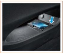
The lower USB charging interface of the console is located above the lower storage tank of the console. It can only work when the Start switch is set to "ON" or "ACC".
