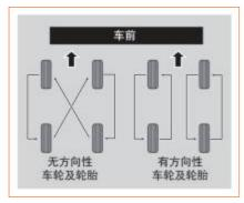
In order to prolong the service life of the tire and make the tire wear evenly, the tire shall be rotated every 10,000 km. Each time of transposition, the operation shall be carried out according to the method shown in the above figure.
