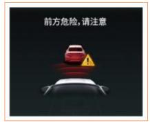
When the AEB system triggers automatic emergency braking, a warning icon will pop up on the combination instrument at the same time, and an audible alarm signal will be given.
