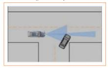
When another vehicle is suddenly cutting in laterally in front of the vehicle, the ACC system may not be able to control the vehicle quickly or apply emergency braking. In this case, the driver shall pay attention to the traffic conditions ahead.
