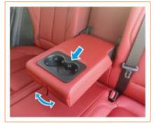
The rear-row central armrest is provided with a cup holder, and the strap can be pulled downward to roll out the cup holder.
