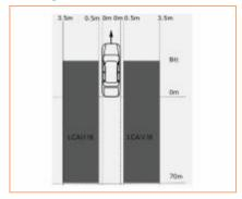
The alarm area of the LCA system is 0.5 m to 3.5m laterally from the left and right sides of the vehicle, and longitudinally from B-pillar to 70 m behind the rear of the vehicle, as shown in the figure. The shaded area is the warning area, which is bilaterally symmetrical.
