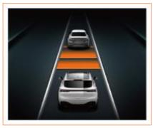
When the following distance is set to be medium, the combination instrument displays as shown in the figure above.
