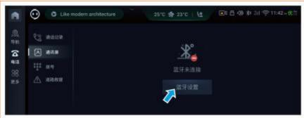
When the Bluetooth switch is not turned on, the Bluetooth phone interface displays Bluetooth setting. Tap Bluetooth setting to jump to the Bluetooth setting interface for detailed operations.
