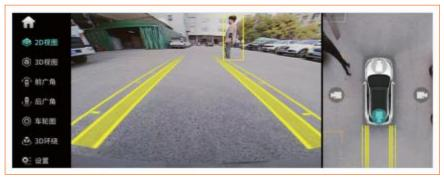
The 4 wide-angle cameras around the vehicle body monitor moving objects in close range in real time.
