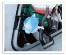
Check whether there is enough washer fluid in the washer fluid reservoir.
