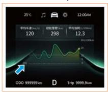
Instantaneous fuel consumption displays the current fuel consumption information through a curve graph.
