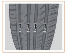
The tire must be kept in good condition, and the tread pattern on the tire surface shall be deep enough. The tire wear degree can be measured by the raised points in the tire driving belt. If the tread thickness is  $\leq 1.6$  mm, the tire must be replaced. Such a tire lacks adhesion when running on wet and slippery roads.
