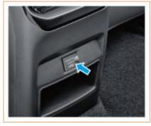
The USB charging interface at the rear row is located below the rear-row air outlet of the console. It can only work when the Start/Stop switch is turned to "ON" or "ACC".
