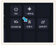
Swipe down on the multimedia display screen and tap "Front radar" to turn on or off the front radar.
