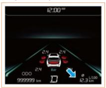
This interface displays the average fuel consumption of the vehicle after last resetting. Display range: 0~19.9 L/100 km.
