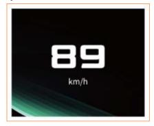
The speedometer displays the current vehicle speed (km/h). Affected by tire pressure, road conditions, climate and other factors, the displayed vehicle speed may deviate slightly from the actual speed.
