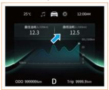
The curve fuel consumption shows the fuel consumption within the last 5 km. The
