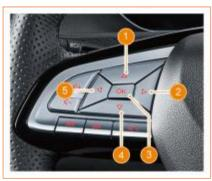
Press the up/down/left/right and OK buttons on the steering wheel to toggle the display in the "Comprehensive Information" area.
