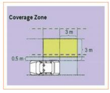
The SVA system can detect an area of about 3 m $\times$ 3 m on the left and right sides behind the vehicle.
