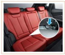
For a child restraint system with ISOFIX interface in the rear seat of the vehicle, the child safety device conforming to ISO standard can be fixed by ISOFIX interface. Please follow the CRS manufacturer's operating instructions and safety prompts during installation and use, as failure to do so may affect the protective effect.
