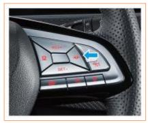
Press the lane keeping assist button to turn on or off the system.
