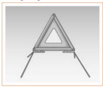
If an accident happens when the vehicle is running, keep to the right as far as possible, take out the warning triangle from the trunk, turn the reflector back to the vehicle and place it at the position of 100~200 meters directly behind the vehicle to remind the oncoming traffic.
