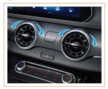
Turn the air outlet switch knob clockwise to close the air outlet, and counterclockwise to open the air outlet. The air direction can be changed by moving the grille in the middle of the air outlet up and down, left and right.
