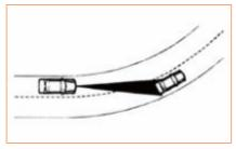
When the vehicle is entering/leaving a curve, the ACC system may respond to vehicles on adjacent lanes and apply brake. This braking process can be ended in advance by depressing the accelerator pedal.
