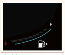
The fuel gauge displays the amount of fuel in the fuel tank in energy block. When the vehicle is turning or running on an uneven road section, the displayed fuel level will slightly deviate from the actual value. If the fuel quantity is small, the low fuel level warning indicator lights up to show that the fuel level in the tank is insufficient and that refueling has to be done as soon as possible.
