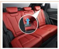
Pull up the locking buckle at the top of the backrest to unlock the seat backrest lock, and then gently fold the seat backrest forward.
