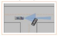
When another vehicle is suddenly cutting in laterally in front of the vehicle, the TJA system may not be able to control the vehicle quickly or apply emergency braking. In this case, the driver shall pay attention to the traffic conditions ahead.
