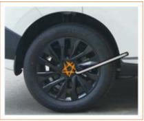
Remove the wheel nuts with a wheel nut wrench, and then remove the tire. Clean the sludge on the hub surface, and then install the spare tire. Tighten the wheel nuts in a crossed sequence as shown in the figure until the wheel is tightly close to the brake hub. Lower the vehicle to the ground and take out the jack. Tighten the wheel nuts in the same cross manner. Then install the nut trim cover with wheel nut cap clip. The specified torque shall be used when tightening the wheel nuts.
