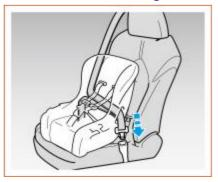
According to the manufacturer's instructions, thread the seat belt through the forward-facing CRS and insert the locking tab into the buckle, ensuring the seat belt is not twisted and remains taut. Confirm that the locking tab and buckle are firmly locked, press the CRS against the seat cushion and seat backrest to fully retract the seat belt, so that the CRS can be fixed firmly, and then check the stability of the CRS by shaking it from side to side.
