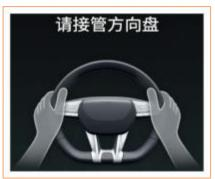
The combination instrument will continuously display the text prompt of "Please take over the steering wheel" with alarm sound at the same time until the user puts the hand on the steering wheel.
