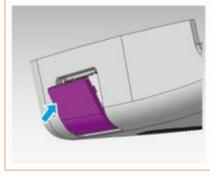
As shown in the figure, pry up the plug with a straight screwdriver at its upper part to take out the TF card. For installation, pre-install the lower end of the plug in place and screw the plug upward to fasten it.
