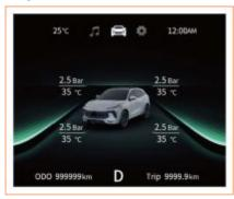
This interface displays the corresponding tire pressure and temperature values. In case of tire abnormality, the display interface will give a corresponding reminder.
