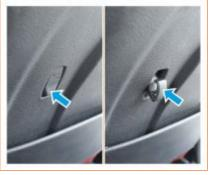
Hooks are designed on the back of front seats for hanging water cups and other light items.
