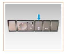
Press the ESP switch, the ESP system will be turned off and the ESP system OFF indicator on the combination instrument will light up.
