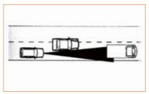
For a vehicle that is not running in the same straight line (a vehicle entering from the adjacent lane), if they do not enter the detection range of the camera sensor, the sensor may not detect that vehicle, resulting in TJA response delay. The driver shall pay close attention to the movement of vehicles in adjacent lanes and take over when necessary.
