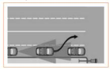
If the vehicle ahead, which is behind a stopped vehicle, suddenly changes to another lane, the system may not have enough time to brake and the driver shall take control of the vehicle if necessary.
