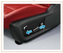
Push the seat forward/backward/height adjustment button gently forward or backward to move the seat forward or backward.
