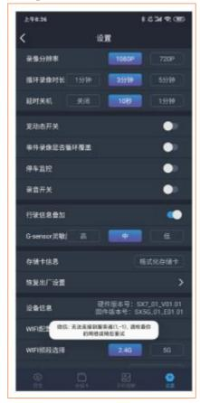
The following is available in "Setting": video recording resolution, video recording duration, delayed shutdown duration, Gsensor sensitivity and WIFI frequency band; enabling or disabling of wide dynamic range (WDR), circular coverage of event video, parking monitoring, audio recording, information superposition and formatting memory card; viewing of device information and WIFI configuration.
