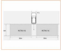
The RCTA system alarm area is 0 m to 30 m laterally from the left and right sides of the vehicle, and longitudinally from the rear of the vehicle to 6 m behind the rear of the vehicle, as shown in the figure. The shaded area is the warning area, which is bilaterally symmetrical.
