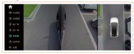
Tap "Wheel diagram" on the left to switch to the corresponding view.
