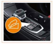
Press the HDC switch, and the HDC system indicator on the combination instrument will light up, indicating that the HDC function is turned on. When the HDC button is pressed again or the vehicle speed exceeds 60 km/h, the HDC system working indicator goes out and the HDC system is turned off.
