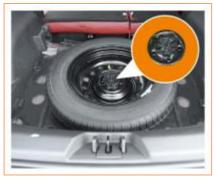
Unscrew the center bolt fixing the spare tire, and take out the spare tire from the spare tire groove.
