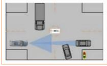
When the target vehicle followed by the subject vehicle passes through an intersection, the driver shall pay attention to the change of traffic lights and take over the vehicle when necessary to avoid violating traffic rules.
