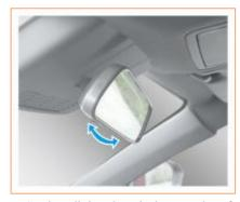
Gently pull the tab at the bottom edge of the interior rearview mirror to switch the mirror reflection state in order to prevent dazzling.
