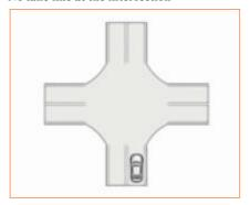
When the vehicle travels to an intersection, the LKA system may exit due to absence of the lane line ahead, or abnormal identification and steering may occur due to the influence of crosswalk and other road markings at the intersection.
