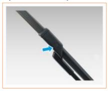
1. Pull up the wiper arm and press the wiper blade release button.
