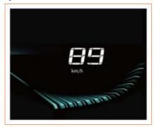
The speedometer displays the current vehicle speed (km/h). Affected by tire pressure, road condition, climate and other factors, an error may occur between the indicated speed and the actual one.
