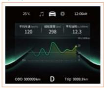
This interface displays the average vehicle speed, endurance mileage, average fuel consumption and instantaneous fuel consumption. The display content can be switched by the up and down buttons on the steering wheel.
