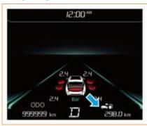
The maximum distance that the vehicle can continue to travel currently is estimated and displayed according to the latest comprehensive fuel consumption and the remaining fuel in the fuel tank.
