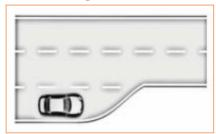
When the vehicle travels to the lane line convergence position, the LKA system may exit because it identifies that the vehicle cannot pass through due to the lane line convergence ahead.
