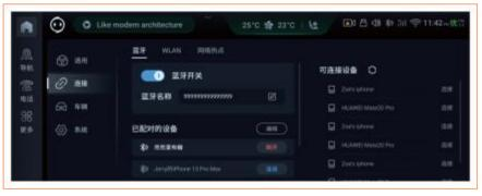
Secondary menu of connection setting: Switch to view and adjust Bluetooth setting/WLAN setting/network hotspot setting, and conduct operations such as Bluetooth connection, WiFi connection and hotspot connection.
