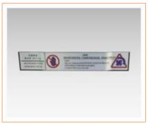
The radiator warning label and the A/C refrigerant label are pasted above the inner side of the engine hood. Coolant specified by Dongfeng Forthing shall be used. Do not mix coolants of different brands. Do not touch the radiator, as the cooling fan may start at any time.
