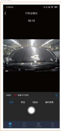
The "Preview" function allows remote control of the dash cam for "video recording", "snap shot", "5-continuous shooting" and "time-lapse photography". Operate the dash cam to take photos and videos and save them in the mobile phone.
