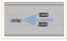
The TJA system cannot accurately judge the width of the lane ahead. When feeling that it is impossible to pass through normally, the driver shall immediately depress the brake pedal to turn off the TJA system and take over the vehicle.
