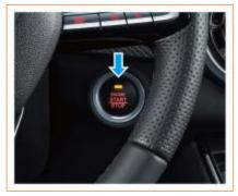
Press the Start/Stop switch without depressing the brake pedal. The Start/Stop switch can be switched between OFF, ACC and ON cyclically.
