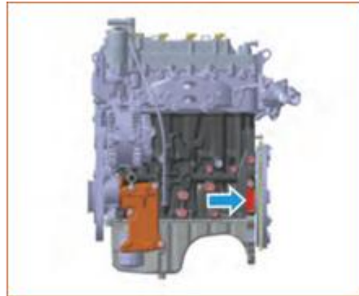
4C16NR Engine number engraving position
