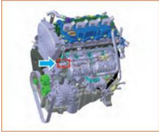
4A92 Engine number engraving position
