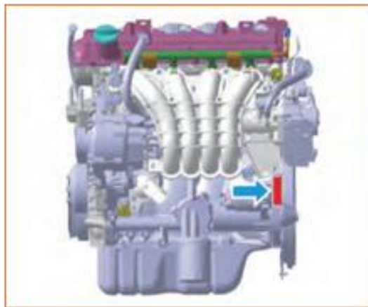
DFMC15TP1 Engine number engraving position
