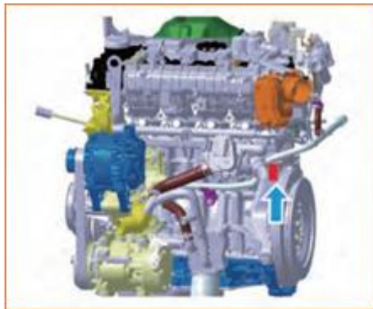
DFMC15TP1 Engine number engraving position
