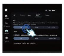
Tap the [Settings] - [Vehicle] - [Driving Assist] - [Lane Change Assistance (LCA)] switch on the display screen in turn to enable or disable it, which is enabled by default. The alarm mode can be selected as "Display" or "Display + Sound", and the vehicle defaults to [Display + Sound].
