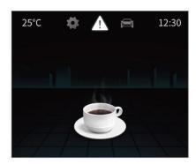
If the fatigue driving reminder will be triggered after continuous driving for more than 4 hours, short press the OK button on the steering wheel and park the vehicle in a safe place for 20 minutes to release the prompt message.
