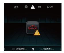
This interface displays some vehicle information that needs to be alarmed or reminded. When there are multiple pieces of information, you can switch and query the displayed contents by pressing the Up and Down keys on the steering wheel.
