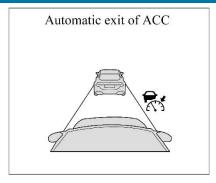
As ACC system cannot provide the maximum braking force of the vehicle, under certain driving conditions, its deceleration capability is not enough to keep a sufficient distance from the vehicle ahead. In these emergencies, ACC system will require the driver to take over the vehicle in time.
