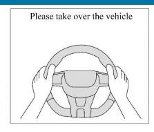
When the TJA system exits, the combination instrument will display a text prompt of [Please take over the vehicle] and buzz at the same time. At this time, the driver needs to take over the vehicle.
