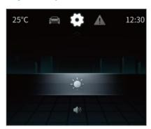
The brightness of the combination instrument backlight can be adjusted. Confirm the information by pressing the up, down and OK keys on the steering wheel; exit the brightness adjustment interface by pressing the left key.
