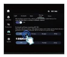
Tap [Settings] - [Vehicle] - [Driver Assistance] - [FCW] switch on the display screen to turn it on or off, and select the functional sensitivity.
