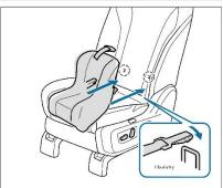
2. Align the ISOFIX interface of the child restraint system with the corresponding ISOFIX interface at the bottom of the seat cushion, inserting the rigid interface and buckling the elastic interface.
