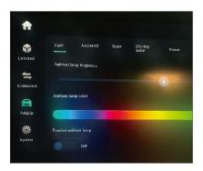
Tap [Settings]-[Vehicle]-[Lighting] on the screen in turn to select the brightness and color of the ambient lamp.
