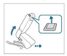
For the middle-row seats of the three-seat model, the left seat can be folded forward as a whole. During operation, place the headrest of the left seat in the middle row to the lowest position, pull the seat folding handle upwards, and push forward and fold the seat. After passengers get on/off the vehicle, fold the seat back, press down and lock it, and slide the seat back to the lockable area to restore the seat to its initial state.
