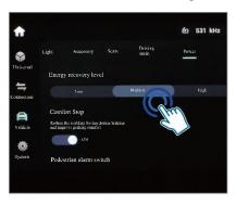
Sliding energy recovery has the effect of braking and deceleration. Tap [Settings] - [Vehicle] - [Power] - [Energy Recovery Level] on the display screen in turn to set sliding energy recovery as a low, medium or high gear according to driving habits. This gear can be memorized automatically. In the gear with weak coasting energy recovery, energy recovery will not be carried out (if deceleration is required, braking energy recovery can also be carried out when the brake pedal is depressed).
