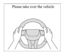
The combination instrument will continuously display the text prompt of [Please take over the vehicle] with alarm sound at the same time.
