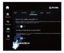
Tap [Settings] - [Vehicle] - [Driver Assistance] - [IHC] switch on the display screen to turn it on or off. It is enabled by default.
