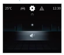
The volume of the combination instrument can be adjusted. Press the Up, Down and OK buttons on the steering wheel to confirm the information; press the Left button to exit the volume adjustment interface.
