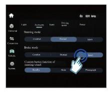
Tap [Settings] - [Vehicle] - [Attachment] - [Braking Mode] on the display screen to select three different modes: comfort, normal and exercise. After the vehicle is restarted, the brake pedal will remember the last set state.
