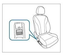
A USB interface is provided inside the middle seat for mobile phone charging.
