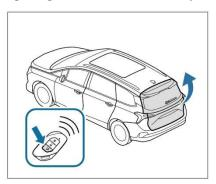
When the trunk lid is closed, press and hold the trunk lid unlock button on the smart key, and the trunk lid will open automatically.
