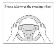
If it is detected that the driver does not hold the steering wheel for a period of time, the combination instrument will prompt "Please take over the steering wheel" with buzzing alarm. At this time, the driver needs to actively take over the steering wheel.
