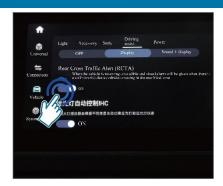
Click [Settings] - [Vehicle] - [Driver Assistance] - [RCTA] on the display screen to turn on or off. It is enabled by default.
