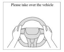
The ACC system will give visual and audible instructions to the driver, and the text prompt [Please take over the vehicle] on the combination instrument will be accompanied by buzzer. In this case, the driver needs to take over the vehicle.
