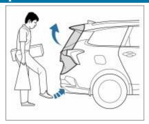
Stand behind the vehicle with the smart key and kick at the middle lower part of the rear bumper. When the kicking action is sensed, the trunk lid will open automatically.
