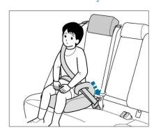
Place the auxiliary cushion on the seat and let the child sit on the auxiliary cushion. According to the instructions provided by the manufacturer, correctly cross the seat belt over the child's shoulder, lower the lap belt as low as possible to the child's hip position, and then insert the latch plate into the buckle to ensure that the seat belt is not twisted and kept tight.
