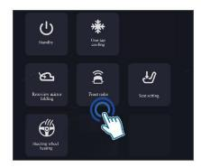
Scribe at the top of the display screen to call out the shortcut menu of the drop-down bar, and tap [Front Radar] to turn on and off the front radar system.
