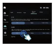
Tap the [Settings] - [Vehicle] - [Driving Assist] -[Door Opening Warning DOW] switch on the screen in turn to enable or disable it, which is enabled by default. The alarm mode can be selected as "Display" or "Display + Sound", and the vehicle defaults to [Display + Sound].
