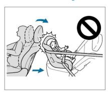
If the rear-facing child restraint system is obstructed by the driver's seat and thus cannot be installed correctly, the rear-facing child restraint system should be installed on the right rear seat.
