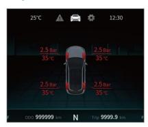
This interface displays the corresponding tire pressure and temperature values. When the tire pressure value is abnormal, the display interface will give a corresponding reminder.
