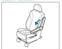
The middle-row seats of the two-seat model have seat armrests, which can be flipped downwards to a fixed position when in three-seat model, the left seat can be folded use and upwards when retracted.
