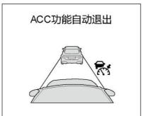
As ACC system cannot provide the maximum braking force of the vehicle, under certain driving conditions, its deceleration capability is not enough to keep a sufficient distance from the vehicle ahead. In these emergencies, ACC system will require the driver to take over the vehicle in time.
