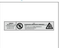
The radiator warning label and the A/C refrigerant label are pasted above the inner side of the engine hood. When replacing the coolant, use the coolant specified by Dongfeng Forthing. Do not mix coolants of different brands. Do not touch the radiator, as the cooling fan may rotate at any time.
