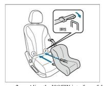
2. Align the ISOFIX interface of the child restraint system with the corresponding ISOFIX interface at the bottom of the seat cushion, inserting the rigid interface and buckling the elastic interface.
