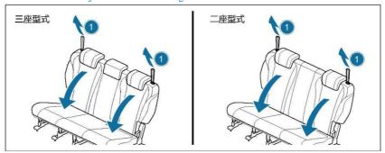
Pull the folding strap of the rear-row seat to adjust the angle of the seat backrest.
