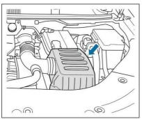
Replace the air filter according to the time and mileage specified in the regular maintenance table. If the air filter is installed improperly, air dust will easily enter the engine, resulting in abnormal wear of the cylinder block. If you need to replace the air filter, please contact the authorized service station of Dongfeng Forthing.
