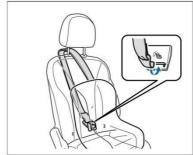
4. Fasten the hook of CRS to the fixed anchor support, and tighten the top
