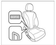
1. Locate the ISOFIX interface position in the gap between the middle-row seat cushion and the backrest.
