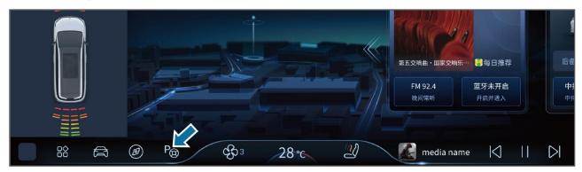
The automatic parking function can be activated by pressing the automatic parking button on the panoramic view interface or at the lower part of the multimedia display screen, or by voice activation on the multimedia display screen interface.
