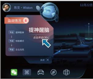
When the driver is severely fatigued, a message will appear on the combination instrument stating "You are driving while fatigued," and a prompt will appear on the multimedia display screen to activate the "Refresh and Alert" mode.
