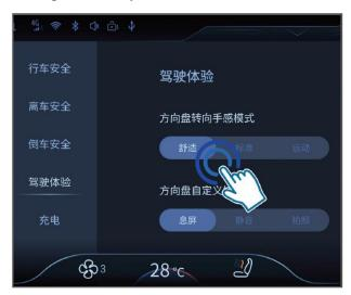
Tap [Vehicle control] - [Vehicle settings] -[Driving experience] - [Steering wheel hand feeling mode] on the multimedia display screen in turn, including three modes: comfort, standard and sport.
