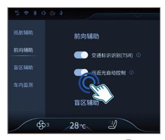
Tap the multimedia display screen [Vehicle control] - [Intelligent driving] - [Forward assistance] - [Automatic control of high and low lights] switch in turn to turn on or off. It is enabled by default.
