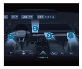
Double click the position of each air outlet 12 34 on the A/C control interface of the multimedia display screen to separately control the opening and closing of each air outlet.
