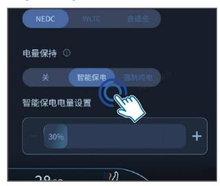
Tap [Vehicle control] - [Vehicle settings] - [Driving experience] - [Battery level holding] on the multimedia display screen in turn to set the battery level sustaining mode as OFF, intelligent power saving or forced pure electric according to driving habits and subsequent road conditions.
