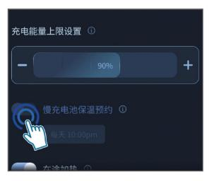
Tap [Vehicle control] - [Vehicle settings] -[Charging] - [Scheduled slow-charge battery thermal insulation] on the home page of the multimedia display screen in turn to enable/disable the traction battery thermal insulation reservation function.
