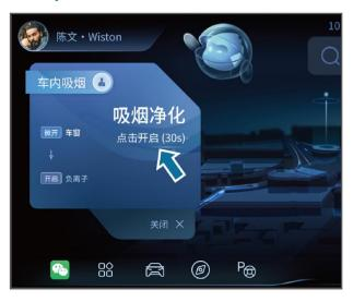
When an occupant is detected to be smoking, the system will actively prompt to turn on the "Smoking Purification" scenario mode to provide a fresh riding environment for the occupants.
