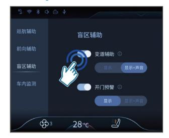
Tap the [Vehicle control] - [Intelligent driving] - [Blind spot assistance] - [Lane change assist] switch on the multimedia display screen in turn to turn on or off, which is enabled by default. The alarm mode can be selected as [Display] or [Display + Sound]. the vehicle defaults to [Display + Sound].
