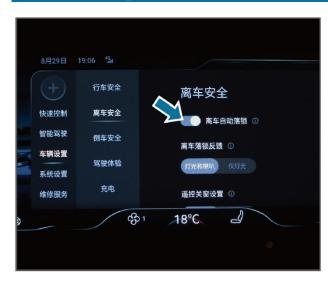
Tap [Vehicle control] - [Vehicle settings] - [Off-vehicle safety] on the multimedia display screen in turn, and select to enable the function of [Automatic locking when off-vehicle]. The off-car locking feedback can be selected from [Lights and horns] or [Only lights].
