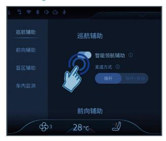
Tap the multimedia display screen [ [vehicle control] - [Intelligent driving] - [cruise assist] - [NOA] switch in turn to turn on or off. The function is disabled by default.
