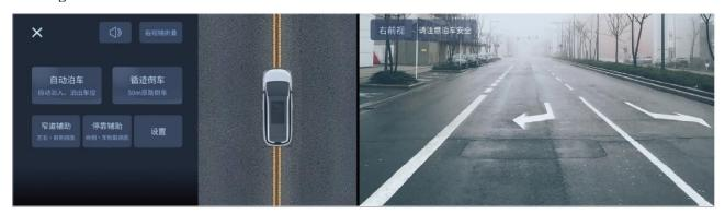
When the steering ON/OFF switch is turned on (not at R position), turn on the left/right turn signal to enter the corresponding left/right turning angle. After pulling the steering lever straight, exit the panoramic view interface with a delay of 1s.
