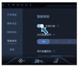
Tap (Vehicle control] - [Vehicle settings] -[Driving experience] - [External light signal] on the multimedia display screen in turn to enable or disable the external light signal function.
