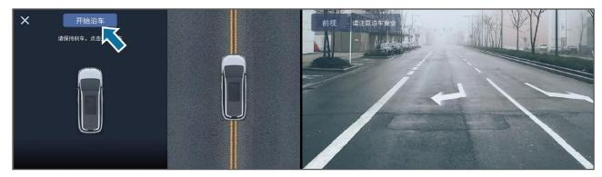
Press the EPB switch, keep depressing the brake pedal, click the [Start parking] button on the multimedia display screen, and release the brake pedal as prompted.
