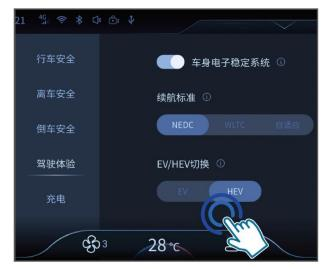
to set two different driving modes: EV and HEV according to driving habits.
