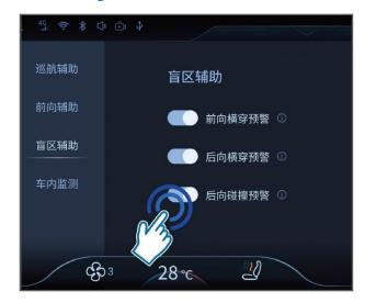
Sequentially navigate the multimedia display screen to access [Vehicle control] - [Intelligent driving] -> [Blind spot assist] - [Rear crossing warning] switch for enabling or disabling. It is set to be on by default.
