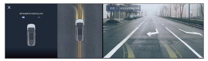
After confirming that the surrounding environment is suitable and safe, select [Automatic parking-out] to enter the automatic parking-out interface, and activate the left or right turn signal according to the prompt to select the parking-out direction.
