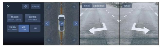
Click the parking assistance button to display the auxiliary view of parking, showing the actual images of the left and right wheels of the vehicle.
