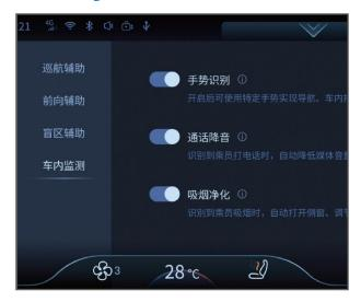
Sequentially navigate the multimedia display screen to access [Vehicle control] - [Intelligent driving] - [In-vehicle monitoring] - [Gesture recognition]/[Voice reduction]/[Smoke purification] switches to enable or disable the corresponding features. Voice reduction and smoke purification are turned on by default.
