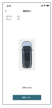
6. After the remote parking-in is completed, the vehicle model and the parking space coincide. Return to the self-test passed interface after 5 s, and click the Exit Parking button to return to the vehicle homepage.
