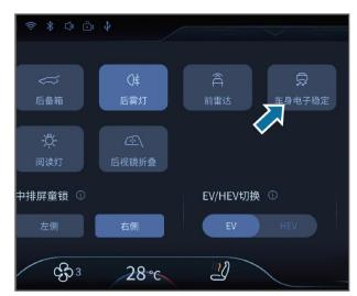
The ESP system is turned on by default. Click [Vehicle control] - [Quick control] - [ESP] on the multimedia display screen in order to turn off the ESP system, and the electronic stability program OFF indicator on the combination instrument will light up.
