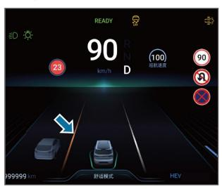
The lane line on the driving interface of the combination instrument is displayed in yellow, and the vehicle deviates towards the yellow lane side. Departure correction will be triggered to provide reverse steering assistance.
