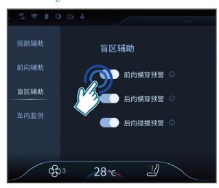
Sequentially navigate the multimedia display screen to access [Vehicle control] - [Intelligent driving] - [Blind spot assist] - [Forward crossing warning" switch for enabling or disabling. It is set to be on by default.
