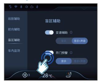
Sequentially navigate the multimedia display screen at to access [Vehicle control] - [Intelligent driving] - [Blind spot assist] - [Door open warning] switch for enabling or disabling. It is set to be on by default. The alarm mode can be selected as [Display] or "Display + Sound], and the vehicle defaults to [Display + Sound].
