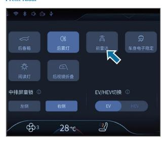
Click [Vehicle control] - [Quick control] - [Front radar] on the multimedia display screen in sequence to turn on and off the front radar system.
