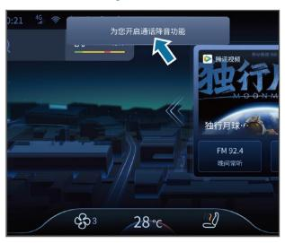
When it is detected that an occupant is making a call, the system will actively turn down the media volume and reduce the air volume of the A/C to provide a quiet communication environment for the occupant.
