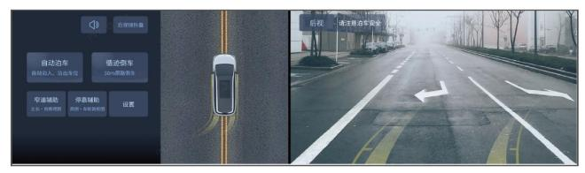
Both the 2D front and rear single view images and the 2D splicing view image have reversing auxiliary lines. The auxiliary lines switch forward and backward with gear D and gear R, and the actual length of the auxiliary line is 5m.
