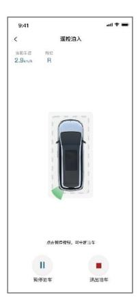
5. After parking is activated, the current vehicle speed, gear position, parking space map and radar signal are displayed. Check whether the vehicle and parking space are consistent with the actual body or click the Pause button to pause parking.
