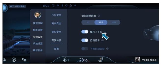
Click [Vehicle control] - [Vehicle settings] - [Driving experience] - [Convenient getting on/off] on the multimedia display screen in turn, and click to enable this function.
