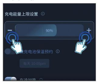
Tap [Vehicle control] - [Vehicle settings] - [Charging] - [Upper limit setting of charging energy] on the home page of the multimedia display screen in turn, and tap [+] or [-] to increase or decrease by 5%, with the adjustable range between  $80\% \sim 100\%$ .
