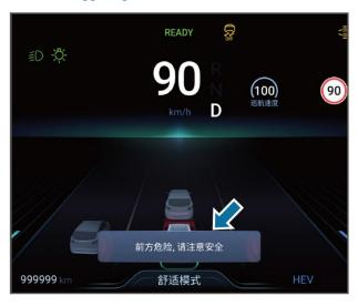
When the FCW is triggered, the front of the vehicle will be marked red on the driving interface of the combination instrument and the text prompts "Danger Ahead, Please Be Careful", accompanied by medium-high frequency alarm sound.
