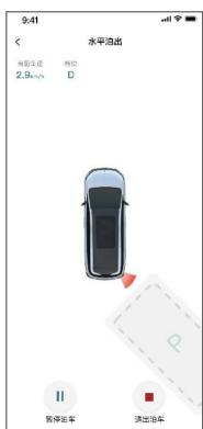
4. After parking is activated, the current vehicle speed, gear position, parking space map and radar signal are displayed. Check whether the vehicle and parking space are consistent with the actual body or click the Pause button to pause parking.
