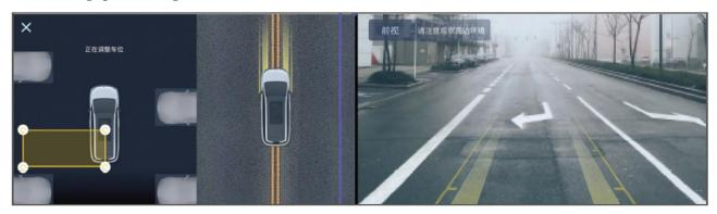
Select "self-selected parking space" on the multimedia display screen or voice "self-selected parking space", and then enter the parking space setting interface. Drag the parking space box on the multimedia display screen to find a parking space available for parking; press and hold the parking space box to drag the adjustment angle at any angle, prompting "Parking Space is being Adjusted". After releasing, it will automatically adjust to vertical, diagonal or horizontal angle.
