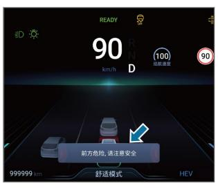
When the automatic emergency braking is triggered, the front of the vehicle will be marked red on the driving interface of the combination instrument, and the text prompts "Danger Ahead, Please Be Careful", accompanied by high-frequency alarm sound.
