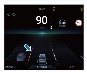
When the vehicle is about to deviate from the lane, the vehicle will give an alarm prompt, and the departure side lane line on the driving interface of the combination instrument will turn red, accompanied by medium frequency alarm sound.
