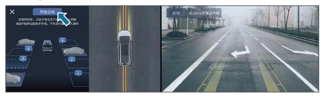
After the vehicle stops, keep braking, confirm that the found parking space and surrounding environment are suitable and safe, click the [Start parking] button on the multimedia display screen, release the steering wheel and brake according to the prompt, and the vehicle starts automatic parking.
