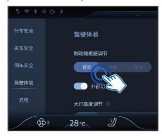
Click [Vehicle control] - [Vehicle settings] - [Driving experience] - [Brake pedal sense adjustment] on the multimedia display screen in turn to select three different modes: Comfort, standard and sport. After the vehicle is restarted, the brake pedal will memorize the last setting state.
