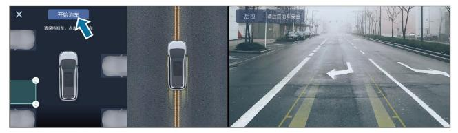
When the parking space box is green, it indicates that the parking space status can be confirmed. After confirming that the parking space and surrounding environment are suitable and safe, click the [Start parking] button on the multimedia display screen, and release the steering wheel and brake according to the prompt.
