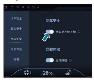
Tap [Vehicle control] - [Vehicle settings] - [Reversing Safety] on the multimedia display screen in turn to enable the function of [Tilting down rearview mirror in reverse]. When the vehicle is reversing, the exterior rear-view mirror can automatically tilt down at a certain angle, which is convenient for the driver to check the road conditions.
