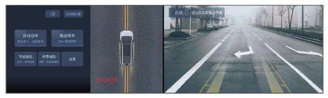
In the panoramic view, automatic parking or trail reversing interface, the alarm is displayed when the corner radar alarm conditions are met.
