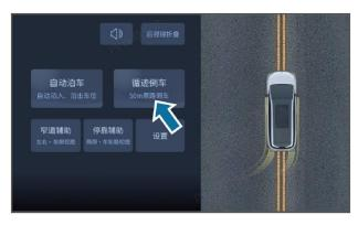
After the vehicle is started, click the "Trail Reversing" button on the panoramic view interface to agree with the disclaimer. The pattern reversing function will be enabled.
