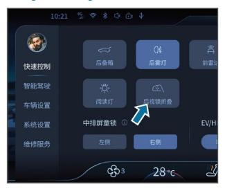
Tap [Vehicle control] - [Quick control] - [Rearview mirror folding] on the multimedia display screen in turn to fold or unfold the exterior rearview mirror.
