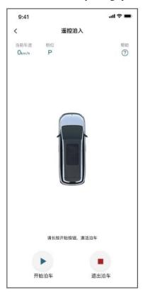
4. After passing the self-inspection, enter the remote parking operation interface. Press and hold [Start parking] for 3 s to start remote parking of the
