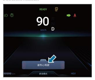
When the system detects that the driver is distracted, the text on the combination instrument will prompt the driver to "Please drive carefully".
