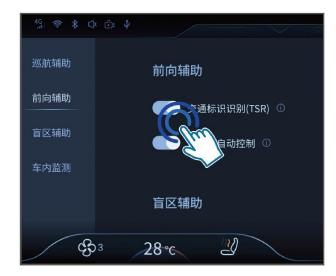
Tap the multimedia display screen [Vehicle control] - [Intelligent driving] - [Forward assistance] - [Traffic sign recognition (TSR)] switch in turn to turn on or off. It is enabled by default.
