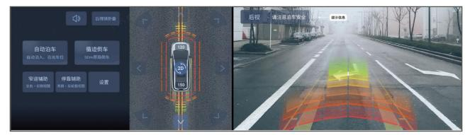
In the panoramic interface, when the working conditions of the radar system are met, the obstacle board will be displayed and an alarm sound will be given.
