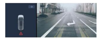
A single radar sensor in front of the vehicle fails, and the other sensors in front do not work. If a single radar sensor behind the vehicle fails, other rear sensors do not work. Please contact an authorized service station of Dongfeng Forthing in time.
