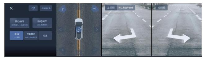
Click the narrow lane assistance button to display the auxiliary view of narrow lane, showing the actual images of left front and right front of the vehicle.
