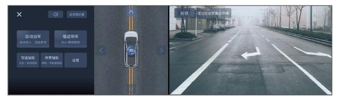
Touch any position of the splicing view to display front, rear, left and right icons. Click it to switch the corresponding angle of view (the icon will be automatically folded if there is no operation for 5 s).
