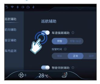
Click the multimedia display screen [Vehicle control] - [Intelligent driving] - [Cruise assist] - [Lane departure assist] switch in turn to turn on or off the system. It is enabled by default. On the premise that the function switch is turned on, you can select the alarm mode as [Warning] or [Warning + Correction]. The default setting is Warning.
