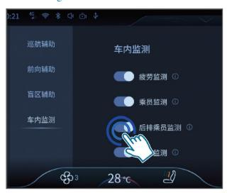
Sequentially navigate the multimedia display screen to access [Vehicle control] - [Intelligent driving] - [In-vehicle monitoring] - [Rear passenger monitoring] switch for enabling or disabling. This switch defaults to the last operation state.
