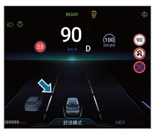
When the lane line on the driving interface of the combination instrument is gray, the LDA function is not activated. When the lane line is white, it indicates that the function is activated.
