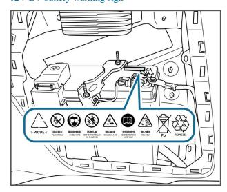
The 12V LV battery warning sign is attached to the surface of the battery. Remind you that the 12V LV battery should be kept away from heat sources and open flames, and ventilation should be maintained during charging and use to prevent accidents.
