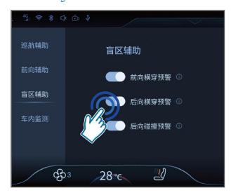
Sequentially navigate the multimedia display screen to access [Vehicle control] - [Intelligent driving] - [Blind spot assist] - [Rear crossing warning] switch for enabling or disabling. It is set to be on by default.
